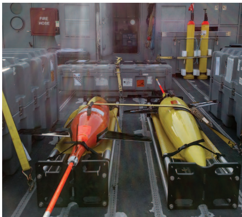
The Seaglider floats are shown in the foreground, and the APEX floats are shown in the rear (upright position). All are equipped with the high performance passive acoustic module.
