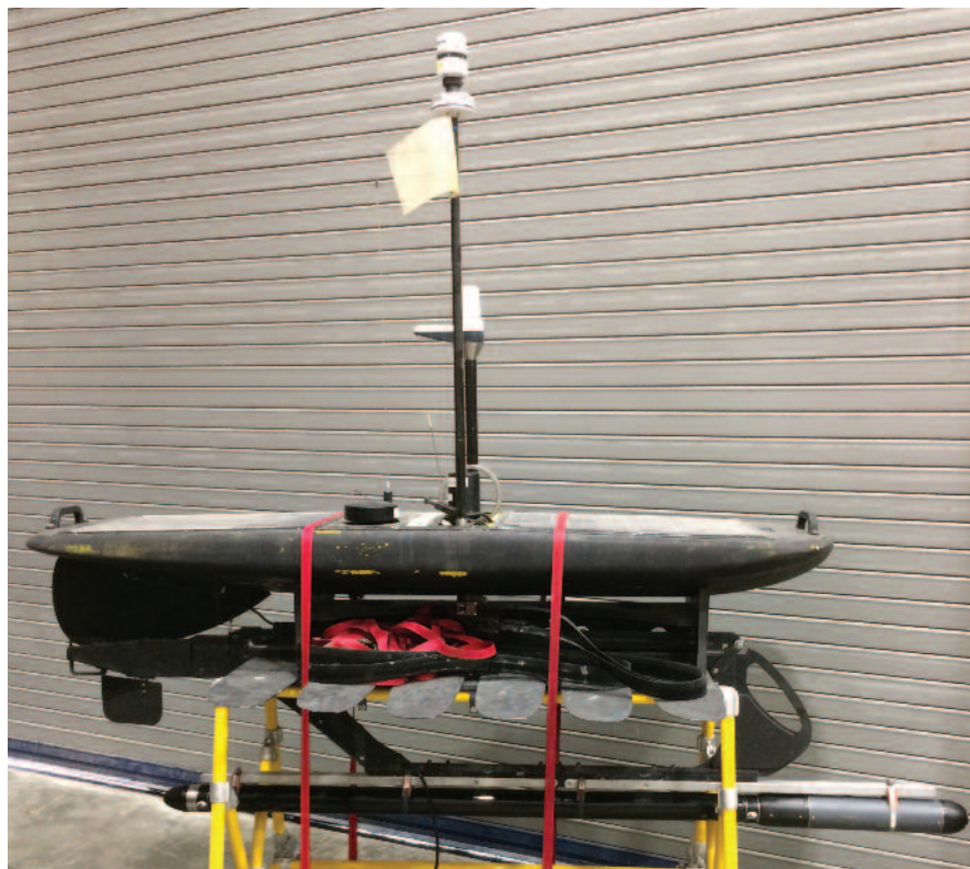
One autonomous platform tested by the project includes a hydrophone array within the black tube at the base of the platform.
