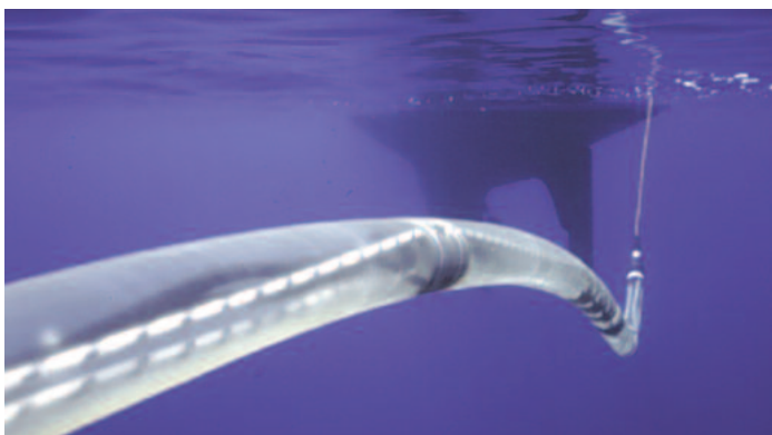
One example of a dipole towed array deployed. D.M. Rossi, University of Pavia
